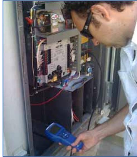
During Acceptance Testing, a technician checks the temperature calibration of a sensor.
